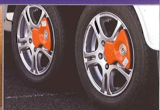
Al-ko Secure wheel clamping system
