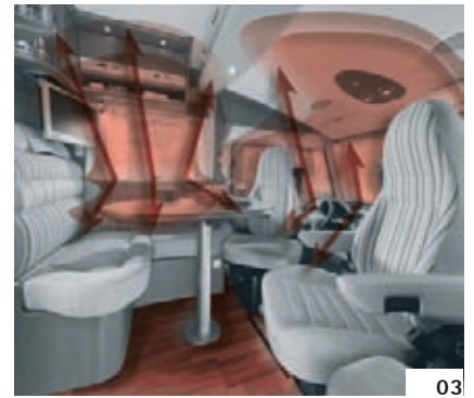
Living space: Hot air outlets at window and under the L-seating group
