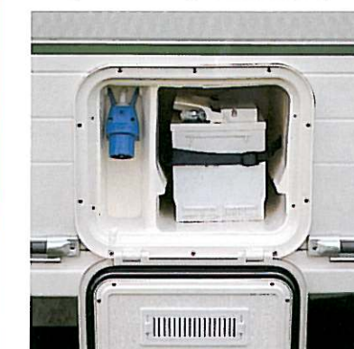
Battery Box with integral mains hook-up
