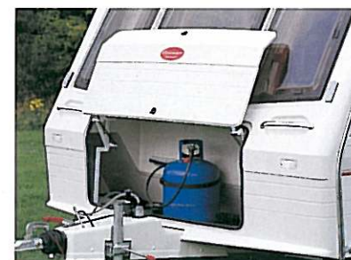
Cantilevered, spring-assisted bottle box door for unrestricted access.
