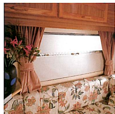
Flyscreens and blinds are built into the main frame of the unique window systems.
