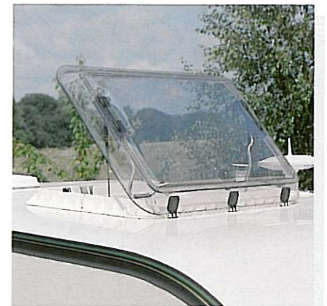
Large tilting panoramic roof window with flynet and blind
