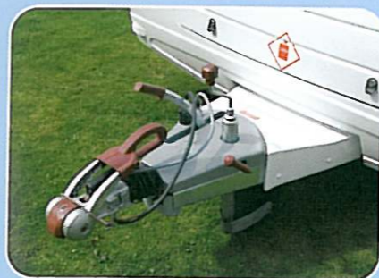
Hitch cover (showing AKS stabiliser fitted to Clubman, Delta, Lexon and Quasar)
