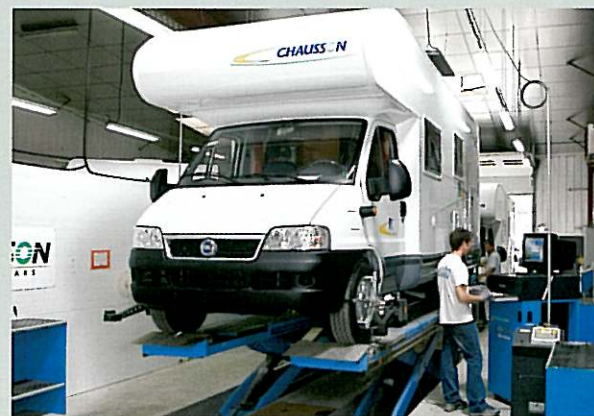
Before delivery, tests are carried out on each Chausson to ensure it is roadworthy. Wheel alignment, unladen weight tests and thorough cleaning.
