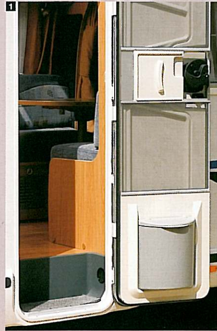
1. Mosquito screen doors with built-in trash can on entire series. (1)
