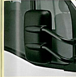
Large exterior rear-view mirrors, with electric de-icing and adjustment. (1)
