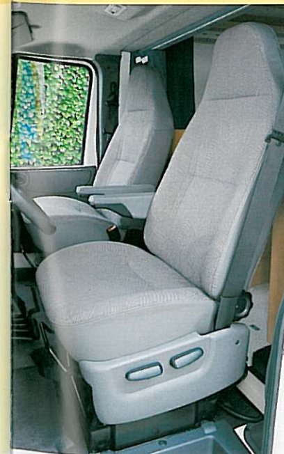
For maximum comfort, the driver's seat can be adjusted forward and backward and up and down. (1)
