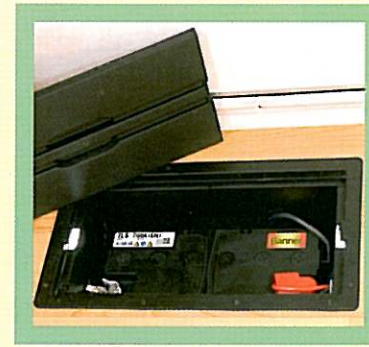
Battery compartment with cover on most models. (1)
