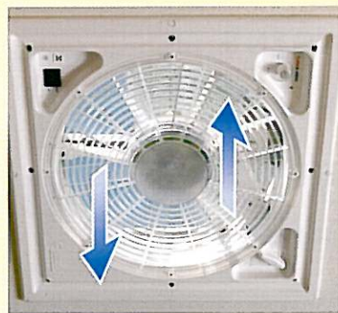
Moon roof ventilator/extractor on all Welcome/Allegro models*. (1)
