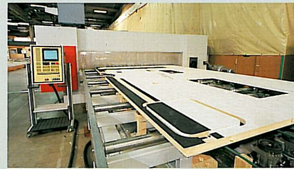
Digital machining center for the manufacture of body panels.
