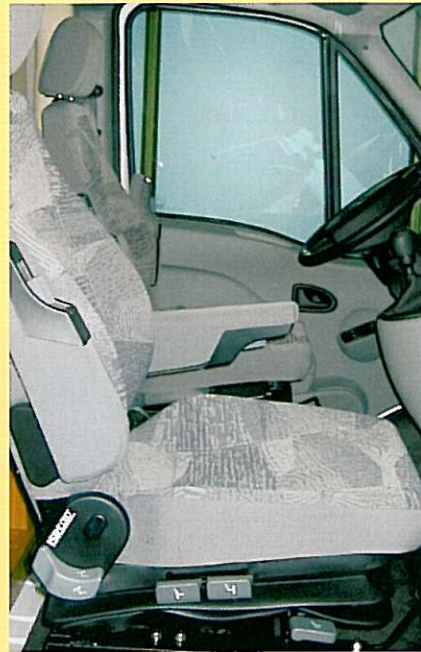
Adjustable seats and handbrake which can be stowed away to allow the seats to be rotated to be used in the panoramic living room. (1)
