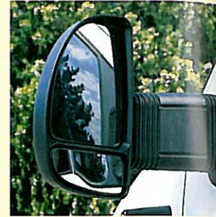
Large exterior, defrosting mirrors that can be adjusted electronically. (1)
