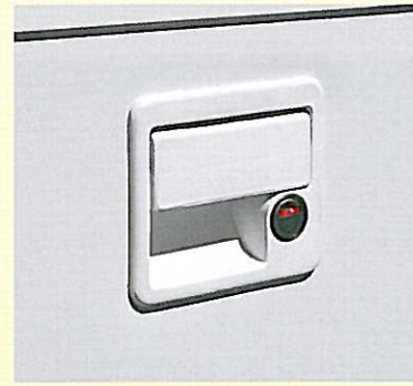
Door locks include grips (except for gas tank door). (1)
