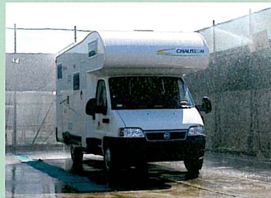
Simulator recreating driving or parking conditions in the rain, which allows a series of sealing tests to be carried out.
