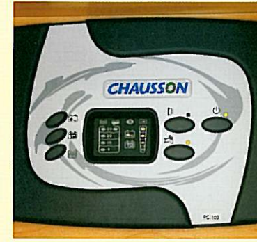
Control system dock with digital display. (1)
