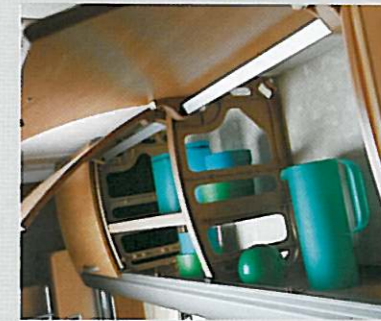
Large upper lockers with spaceframe construction
