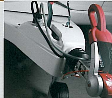
Hitch and A-frame cover with AKS 3004 stabiliser
