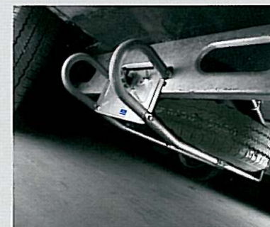
Spare wheel (steel) and underslung carrier
