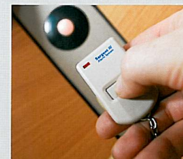
Passive infra-red alarm system with tilt sensor and key fob operation
