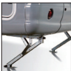
Rear corner steadies fitted as standard to all Cheyenne and Frontier models.
