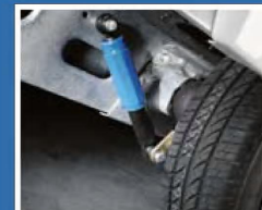
Shock absorbers give more stable, smooth towing
