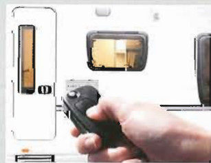
Central locking New high specification entrance door with remote central locking
