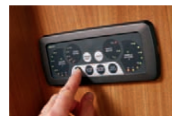
Control Panel The 12V control panel controls the 12V power on/off, water pump and lighting circuits, tank levels and leisure battery state
