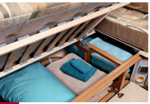
Beech slat seat bases provide comfortable seating whilst sprung hinged tops provide easy access to under seat storage
