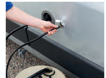
<< 12 volt exterior power point for pump filling of water tank (pump not supplied)
