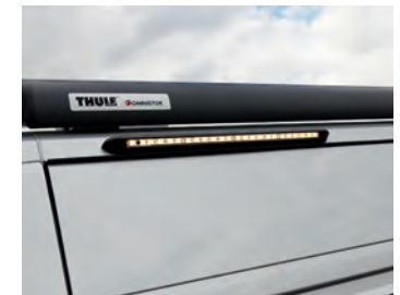
<< New Rain diverter over side entrance door and LED entrance light
