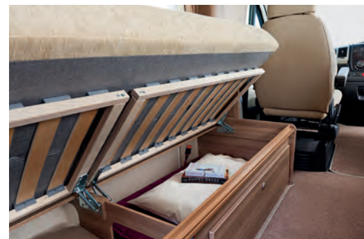
⌘ Seat bases with spaceframe construction, full front access and space for larger items
