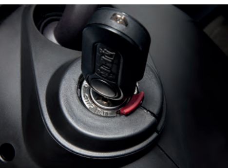
⚡ New: Cab battery isolation switch to prevent discharge in storage
