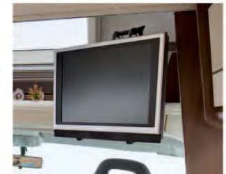
LCD TV provision for TV stand with extractable arm for viewing from the dinette and from the bed in the intermediate and low position.
