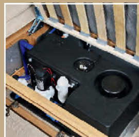
⌘ 30 litre internal fresh water tank with additional pump for tank filling or direct feed to taps
