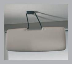
Best guard against dazzling light: For a safe journey even when the sun is low in the sky, both seats in the cab are equipped with flexible sun visors. The visors attached to the pull-down bed can be adjusted for any sunlight intensity via two pivot points.
