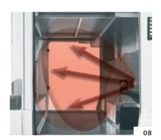
Exterior stowage compartments: Hot air in maxi stowage compartment and garage.
