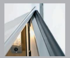
No chance of moisture: All of the vehicle doors and also all of the exterior stowage compartment flaps and doors are protected against rain and spray water by additional spray water seals. This means that there is no chance of water ingress between the door and frame and nothing will freeze shut in the cold.
