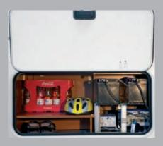
Heated exterior stowage compartments: Both the huge garage in the rear and also the stowage compartment beneath the lounge bench seat are supplied with hot air from the heating system. In this way, cold-sensitive objects and items of luggage can be stored there without worry.
