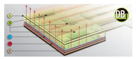
Versatile multi-purpose double floor: Combined in an ideal way by the multi-purpose floor of the Hymermobil B-Class are warmth, security, stability and stowage space. Integrated in the extra strong, 3 cm thick flooring (A) are a wide range of heated storage compartments (B) that can be utilised conveniently from the inside
