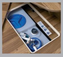
Clear route to fresh water: Likewise in the interior of the vehicle under an additional floor flap is the access point to the fresh water tank. The rotary knob to open and close the overflow has a central location and the large flap is ergonomically formed.
