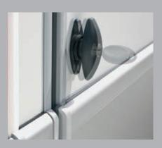
Safe and secure from outside: All of the exterior stowage compartments feature sturdy, ergonomic rotary knobs that ensure optimal closing security. The first 180 degree turn closes the door and an additional 180 degree turn presses the door into the frame with a tight and flush fit.
