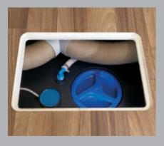
Direct access to the tank: Checking and cleaning the grey water tank is also especially easy and convenient. The cover of the tank is located directly beneath the floor flap and can be accessed with ease from the interior.
