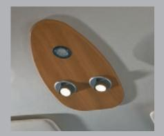
More light on the road: Two bright LED reading lamps supply the cab if required with good lighting during a journey. The spotlights integrated in the furniture are attached to the underside of the pull-down bed and can be switched on from the driver and front passenger seat with ease.
