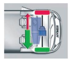
Traction Plus: In conjunction with ESP, this system ensures greater traction on difficult terrain by distributing the torque to the front wheels in a targeted manner. This makes it easier to drive-off on wet grass, for example, or manoeuvre over muddy ground.
