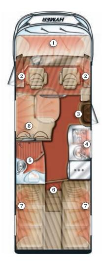
Comfortable, well-balanced heat distribution: The heated multi-purpose double floor works like a complete underfloor heating system in the interior.
