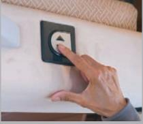
Electric drop-down bed: The 1.50 metre wide drop-down bed above the cab can be raised and lowered electrically with no effort whatsoever. The switch for the jolt-free electric drive is integrated on the front of the bed and can be reached from the living space with ease.
