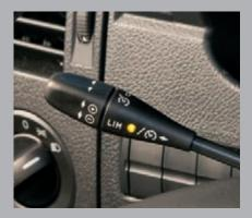
Driving comfort with cruise control: Comfortable and safe at a steady, controlled speed – the onboard cruise control system makes this possible. If the set speed is exceeded, the integrated Speedtronic alerts the driver.
