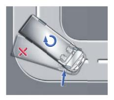
Electronic stability program (ESP): In critical situations, skidding or breaking out of the vehicle is prevented by engine speed adjustment and by targeted braking of individual wheels.
