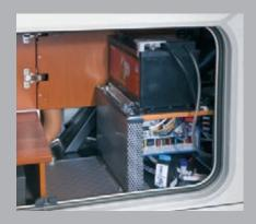
Secure power supply: The powerful AGM leisure battery with 95 Ah is located close to the heater in the heated stowage compartment under the seating group and, if required, can also be extended to two units with additional charger. This means that sufficient power can be supplied safely even at constant low temperatures.
