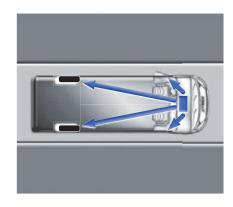
Electronic brake pressure distribution (EBD): This system apportions the brake force optimally to both axles depending on the situation. In this way, the greatest possible braking force is achieved and, at the same time, the vehicle is prevented from breaking out through "overbraking" at the rear.
