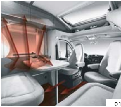
01 Living area: Hot air outlets at the window of the seating group and under the seats in the driver's cab
