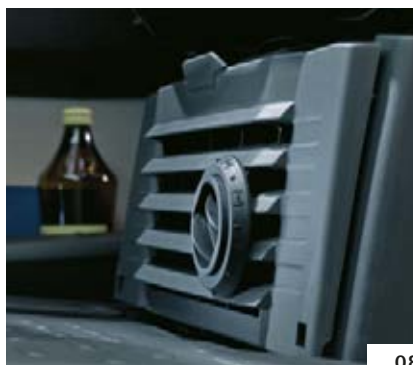
08 Additional heat in the driver's cabin: Heating outlets are located underneath the driver's cabin seats that ensure that the driver's cabin is ideally heated, even when stationary and the vehicle is being used solely for accommodation.
